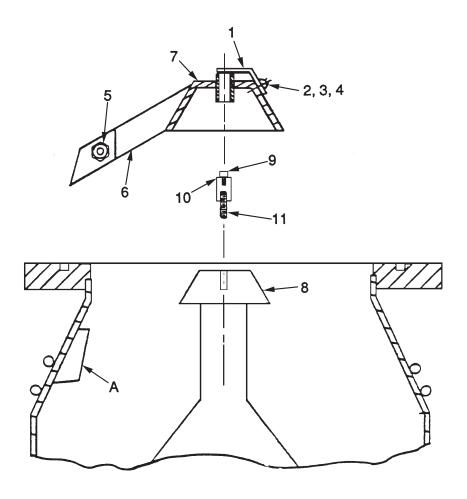
Figure 3-1 Cold Cap Removal/Installation
