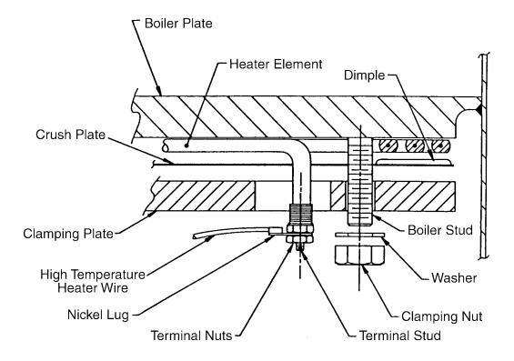
Figure 3-2 Heater Connections, VHS-10 and VHS-400 Pumps
