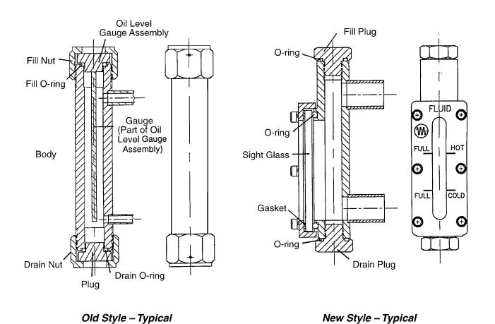
Figure 5-5 Fill and Drain Assemblies
