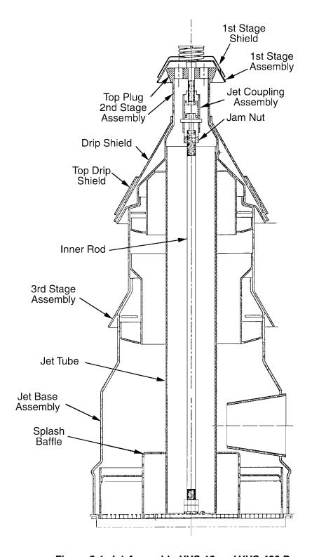
Figure 3-1 Jet Assembly, VHS-10 and VHS-400 Pumps
