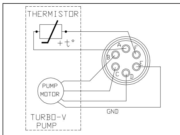
The turbopump is connected to the controller through an 6-pin connector. Pins B, C and D are the 3-phase supply to the motor, pins A and F are connected to the temperature sensor (NTC type, 30 K $\Omega$  resistance at 25° C) and pin E is connected to the pump ground.
