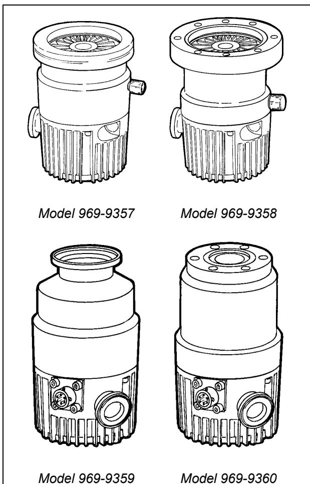
The Turbo-V70 pump consists of a high frequency motor driving a turbine fitted with 11 bladed stages. The turbine rotates in an anticlockwise direction when viewed from the high vacuum flange end.
