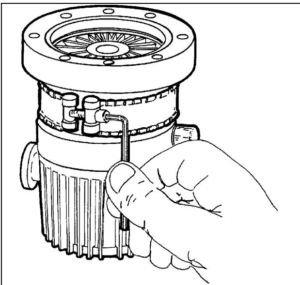
Switch on the heater while the turbopump is in operation. If, for any reason, the turbopump body overheats, it will be automatically cut out by the thermistor sensor.
