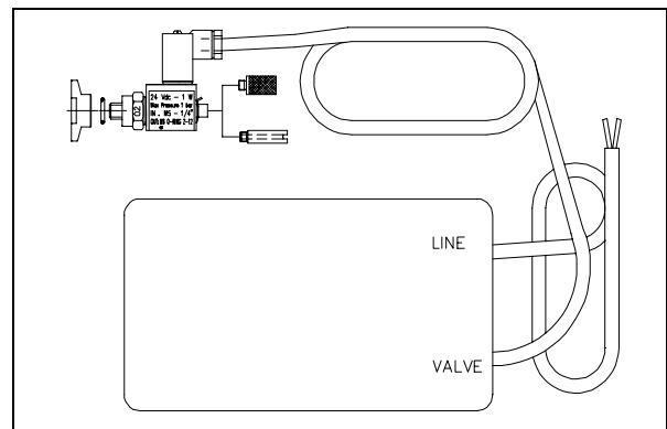
The vent device mod. 969-9831 allows to avoid undesired pump aeration of the pump during a temporary power failure (adjustable time up to 36 min.), and enables an automatic vent operation.
