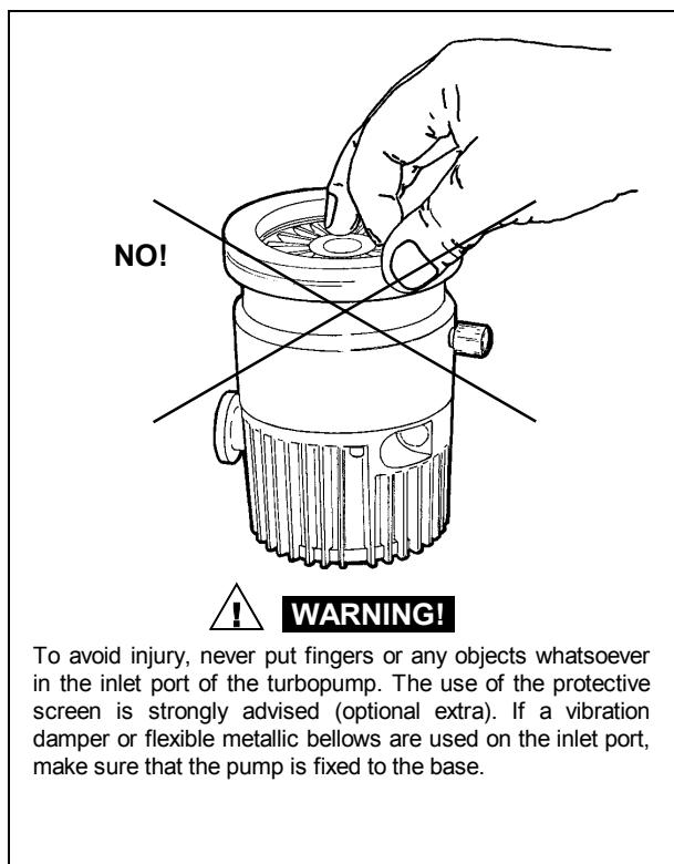
To avoid injury, never put fingers or any objects whatsoever in the inlet port of the turbopump. The use of the protective screen is strongly advised (optional extra). If a vibration damper or flexible metallic bellows are used on the inlet port, make sure that the pump is fixed to the base.
