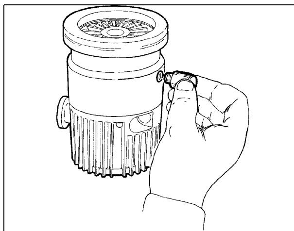
Screw the flange mod. 969-9109 on the pump, taking care of the o-ring right position.
