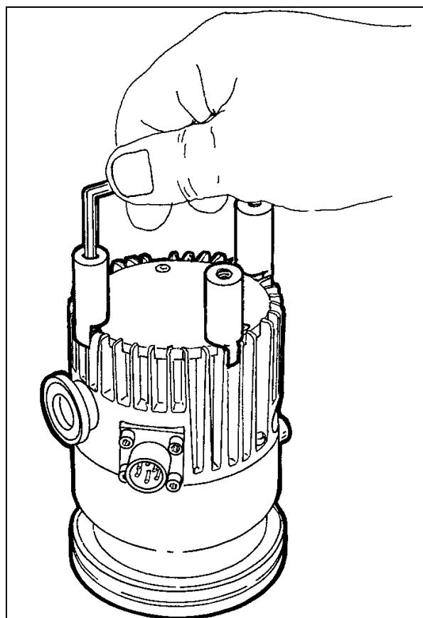
Turn the pump the right way up. Fix the pump to a base by using the three screws provided (M4 thread) in the holes in the three feet.
