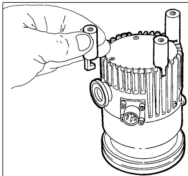
Fix the feet to the pump by tightening the previously inserted grub screws with the Allen key.
