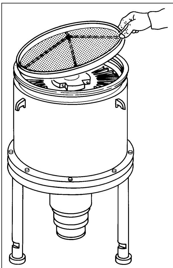
The screen can be mounted on each pump model.
