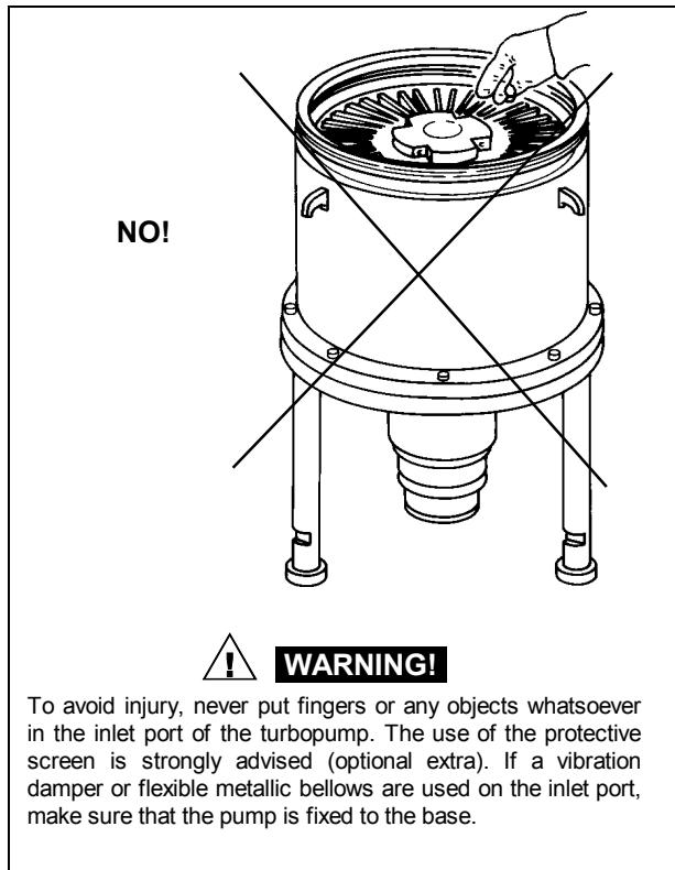
The Turbo - V 6000 series pumps must only be used with one of the special Varian controllers (series 969-9491, 969-9591) and must be connected to a primary pump (see "Technical Information").
