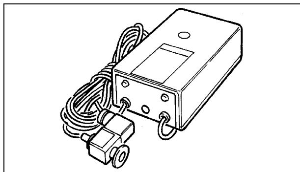
The vent device mod. 969-9831 allows to avoid undesired venting of the pump during a temporary power failure (adjustable time up to 36 min.), and enables an automatic vent operation.
