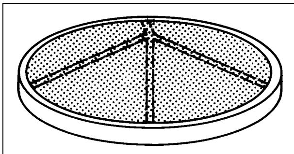
The inlet screens mod. 969-9308 prevents the blades of the pump from being damaged by debris greater than 2 mm diameter.
