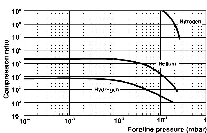
*Graph of compression ratio vs foreline pressure*
