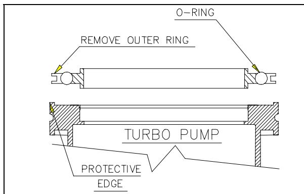
Then fix the two flanges with the clamps or claws as shown in the figure.
