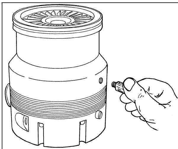
Screw the flange mod. 969-9109 on the pump, taking care of the o-ring right position.
