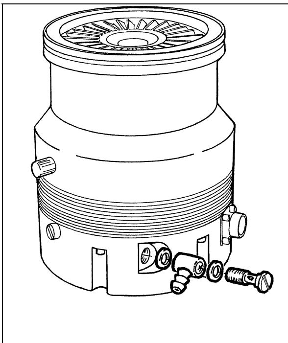
Two 6 mm (1/4") internal diameter rubber or plastic hoses from the water supply must be fitted to the two nozzles.
