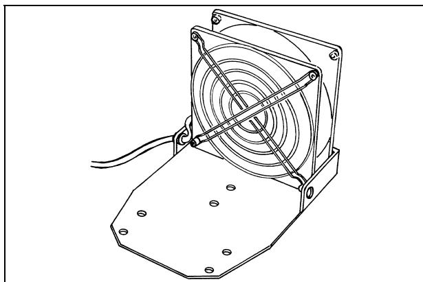
A fan kit model 969-9314 is available for air cooling the pump.
