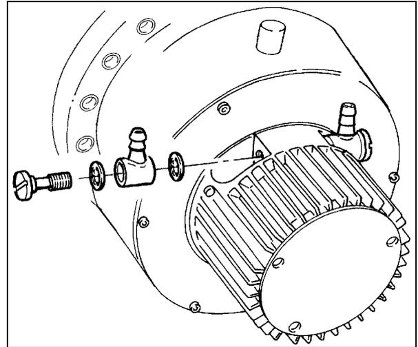
Two 6 mm (1/4") internal diameter rubber or plastic hoses from the water supply must be fitted to the two nozzles.
