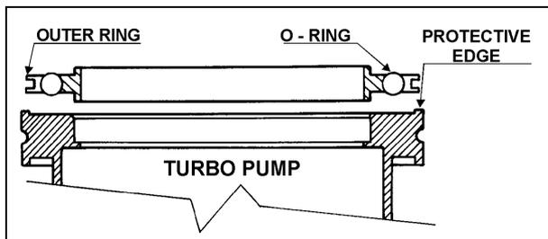
Then fix the two flanges with the clamps or claws as shown in the figure.
