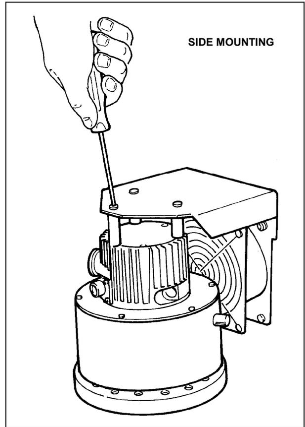
The low power fan can also be mounted under the pump as shown in the following figure.
