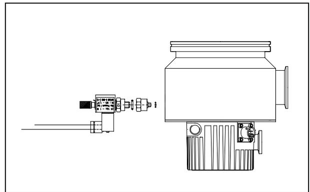
Tighten the valve using a 16 mm hexagonal spanner.
