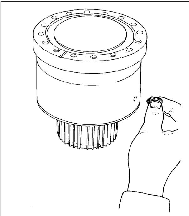
Screw the vent valve into the pump.
