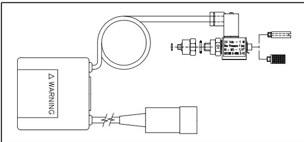
The vent valve mod. 969-9833 enables undesired venting of the pump during a temporary power failure (5 sec maximum) to be avoided, and enables an automatic vent operation.
