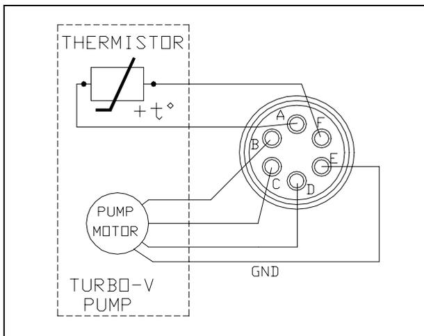
The turbopump is connected to the controller through an 6-pin connector. Pins B, C and D are the 3-phase supply to the motor, pins A and F are connected to the temperature sensor (NTC type, 30 KΩ resistance at 25° C) and pin E is connected to the pump earth.
