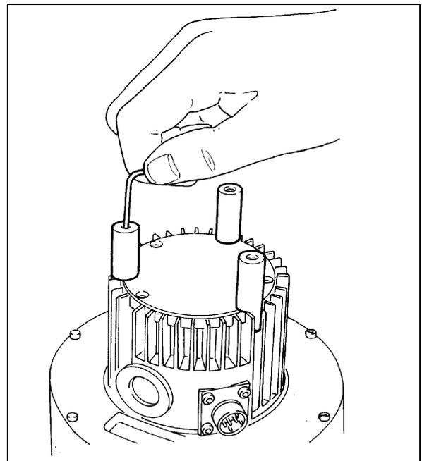
Turn the pump the right way up. Fix the pump to a base by using the three screws provided (M4 thread) in the holes in the three feet.
