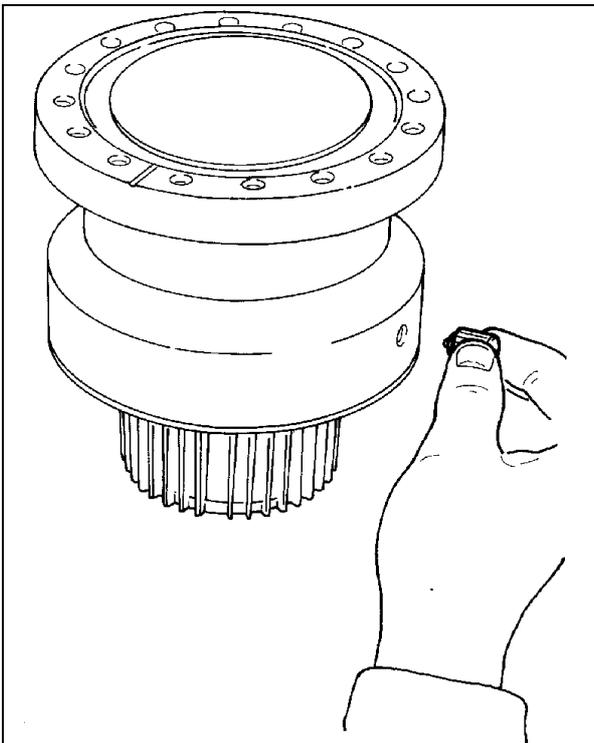
Screw the vent valve into the pump.
