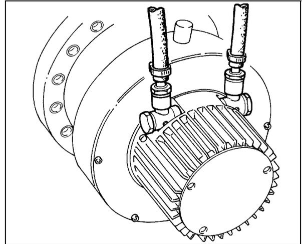
Cooling may be carried out either through an open circuit with eventual discharge of the water, or using a closed circuit cooling system.
