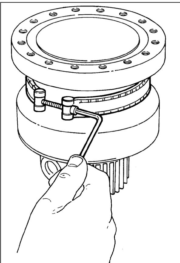
Switch on the heater while the turbopump is in operation. If, for any reason, the turbopump body overheats, it will be automatically cut out by the thermistor sensor.
