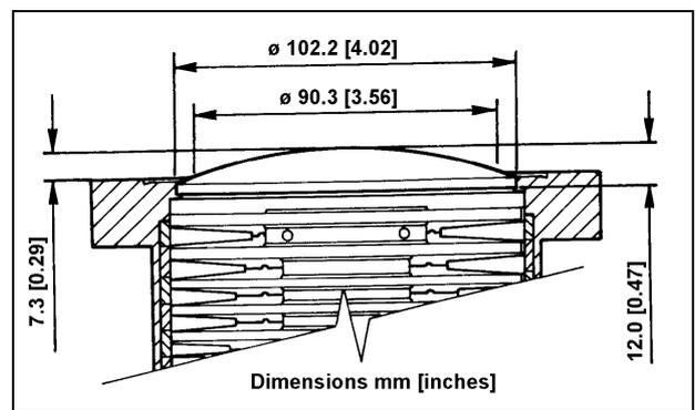
Overall dimensions with the inlet screen fitted on pump series 969-9008 (with ConFlat 6" flange).
