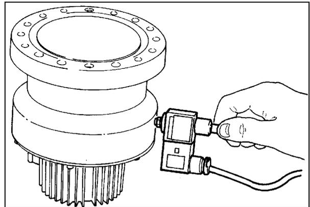
Tighten the valve using a 10 mm hexagonal spanner.
