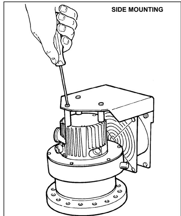
The low power fan can also be mounted under the pump as shown in the figure.
