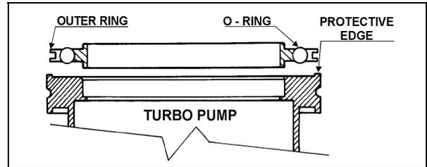
Then fix the two flanges with the clamps or claws as shown in the figure.
