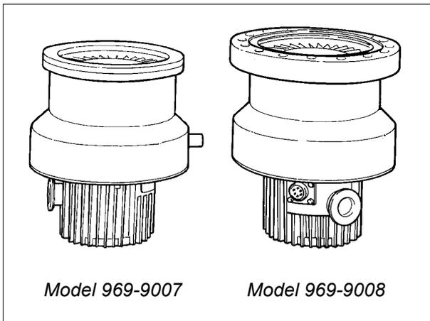
The Turbo-V250 pump consists of a high frequency motor driving a turbine fitted with 8 bladed stages and 3 Macrotrorr stages. The turbine rotates in an anticlockwise direction when viewed from the high vacuum flange end.
