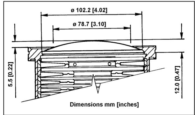
Overall dimensions with the protection screen fitted on pump series 969-9007 (with ISO 100 flange).
