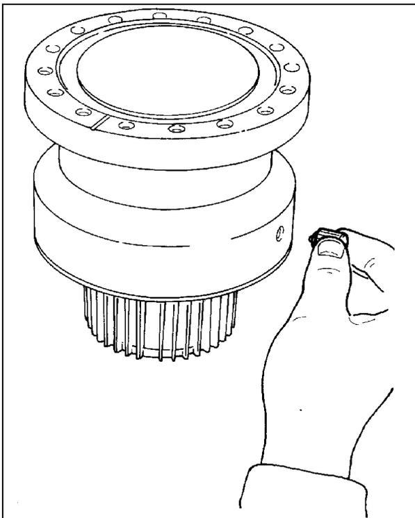
Screw the flange mod. 969-9109 on the pump, taking care of the o-ring right position.
