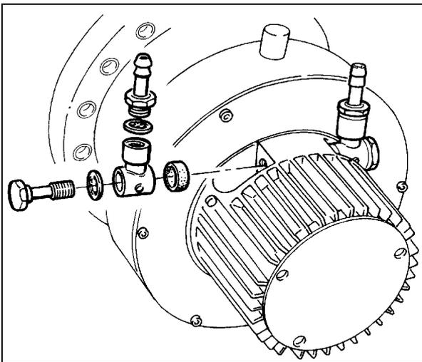
Two 6 mm (1/4") internal diameter rubber or plastic hoses from the water supply must be fitted to the two nozzles.
