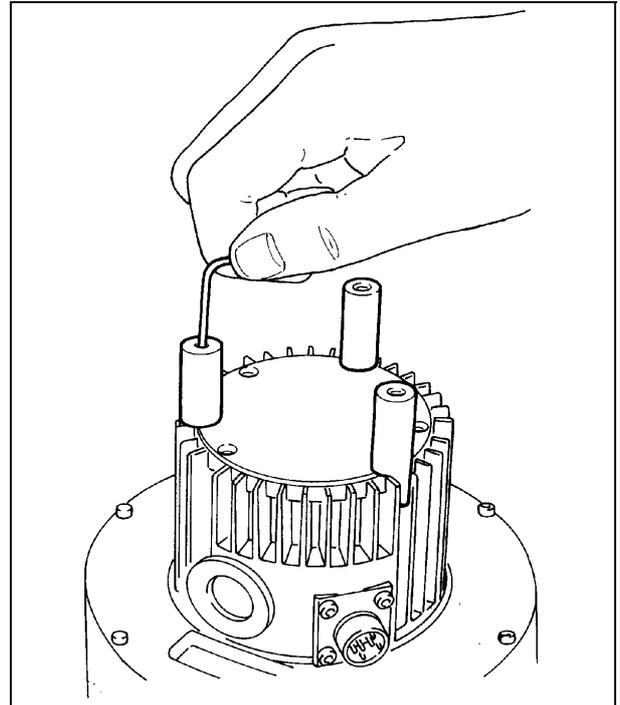
Turn the pump the right way up. Fix the pump to a base by using the three screws provided (M4 thread) in the holes in the three feet.
