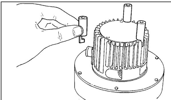
Fix the feet to the pump by tightening the previously inserted grub screws with the Allen key.
