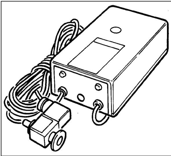
The vent device mod. 969-9831 allows to avoid undesired pump aeration of the pump during a temporary power failure (adjustable time up to 36 min.), and enables an automatic vent operation.
