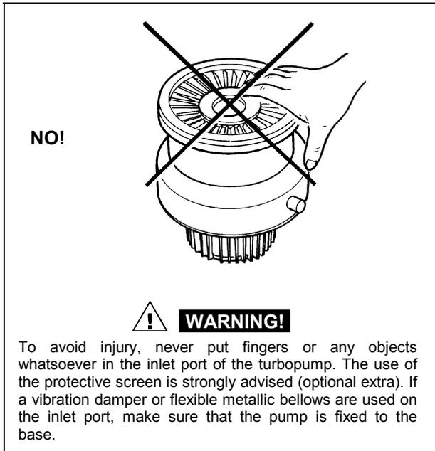
The turbopump with ISO inlet flange must be fixed to the vacuum chamber by means of clamps or claws. The following table shows, for each flange and fixing device, the necessary number of clamps or claws and the relevant fixing torque.
