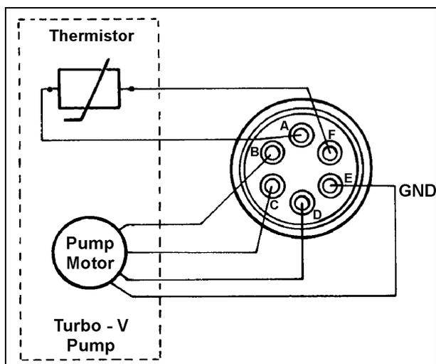
The turbopump is connected to the controller through an 6-pin connector. Pins B, C and D are the 3-phase supply to the motor, pins A and F are connected to the temperature sensor (NTC type, 30 KΩ resistance at 25° C) and pin E is connected to the pump earth.
