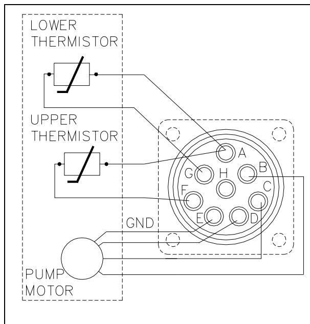
The turbopump is connected to the controller through an 8-pin connector. Pins B, C and D are the 3-phase supply to the motor, pins A and F are connected to the upper bearing temperature sensor, pins A and G are connected to the lower bearing temperature sensor and pin E is connected to the pump ground; pin H is not connected.
