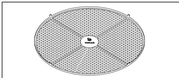
The inlet screens prevents the blades of the pump from being damaged by debris greater than 3 mm diameter. The inlet screen, however, will reduce the pumping speed by about 20%. The inlet screen is fitted in the upper part of the pump, as shown in the figure and can be mounted on each pump model.
