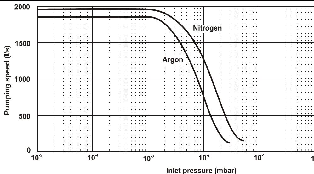
Graph of nitrogen pumping speed vs inlet pressure
