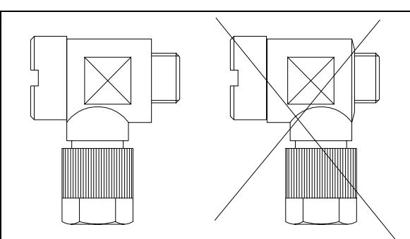
The assembled kit must be screwed into the suitable holes of the pump body with a recommended closing torque of 5 Nm.
