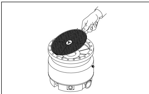
The following figure shows the pump flange sections with the protection screen fitted on them. As you can see, the overall dimensions do not change as the inlet screen remains inside the pump profile.
