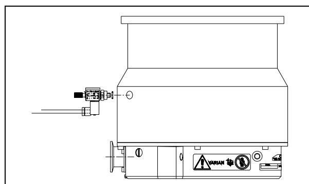
Tighten the valve using a 16 mm. hexagonal spanner with a torque of 2.5 Nm.
