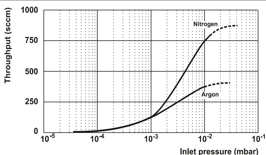
Graph of nitrogen throughput vs inlet pressure using the recommended mechanical forevacuum pump
