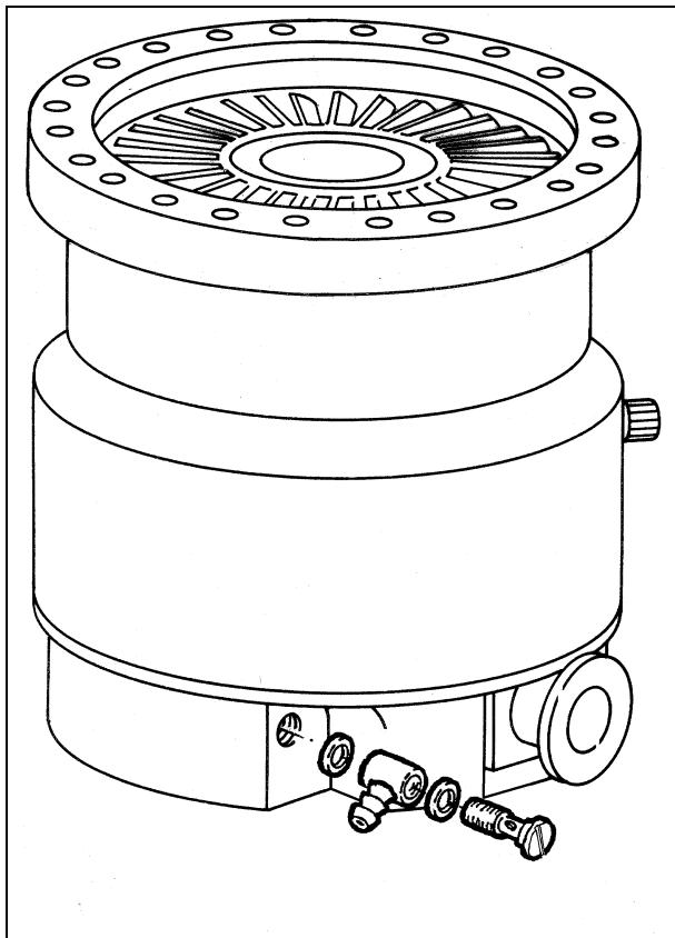
Two 6 mm (1/4") internal diameter rubber or plastic hoses from the water supply must be fitted to the two nozzles.
