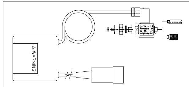
The vent valve mod. 969-9843 allows to avoid undesired venting of the pump during a temporary power failure (5 sec maximum), and enables an automatic vent operation.
