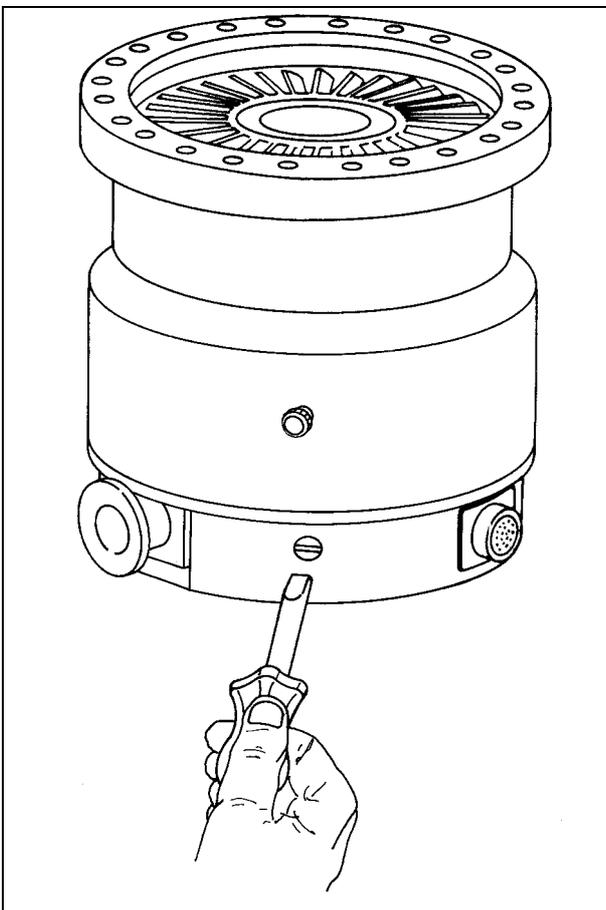
and then screw the gas purge valve (with a torque of 2.5 Nm) as shown in the following figure.
