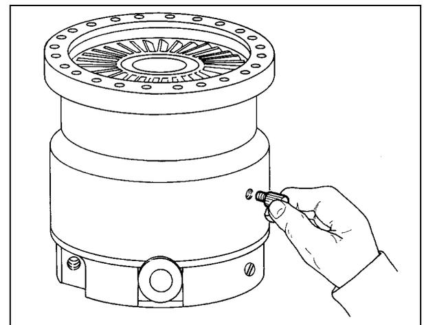
Screw the vent valve into the pump without inserting the supplied adapter between the valve and the pump.
