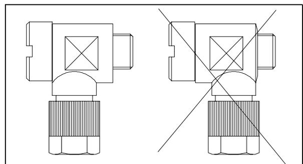
The assembled kit must be screwed into the suitable holes of the pump body with a recommended closing torque of 5 Nm.
