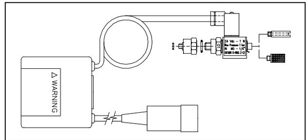
The vent valve mod. 969-9843 allows to avoid undesired venting of the pump during a temporary power failure (5 sec maximum), and enables an automatic vent operation.
