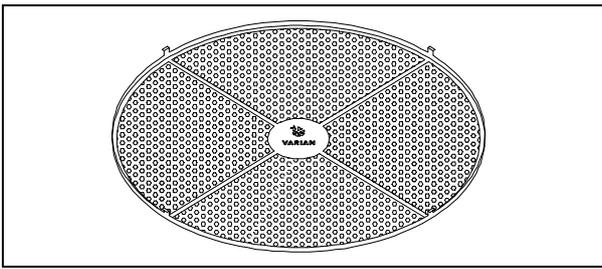
The inlet screens prevents the blades of the pump from being damaged by debris greater than 3 mm diameter. The inlet screen, however, will reduce the pumping speed by about 20%. The inlet screen is fitted in the upper part of the pump, as shown in the figure and can be mounted on each pump model.
