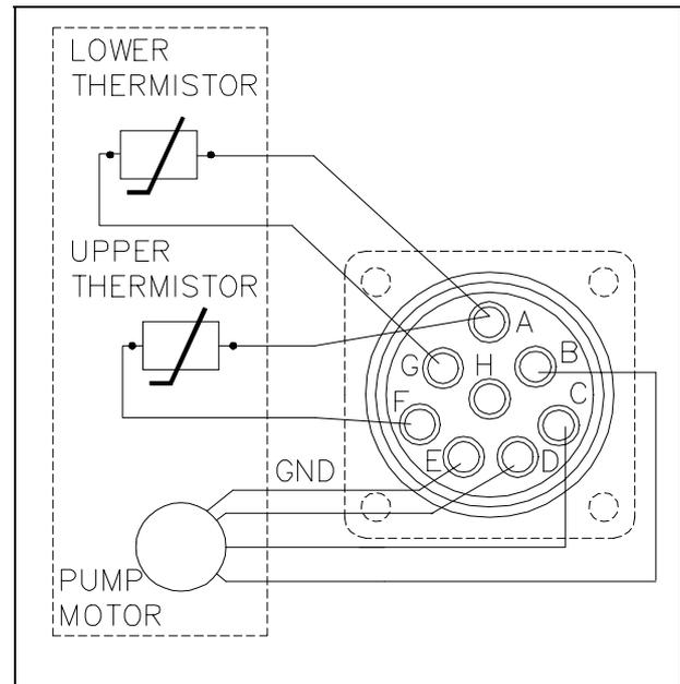
The turbopump is connected to the controller through an 8-pin connector. Pins B, C and D are the 3-phase supply to the motor, pins A and F are connected to the upper bearing temperature sensor, pins A and G are connected to the lower bearing temperature sensor and pin E is connected to the pump ground; pin H is not connected.
