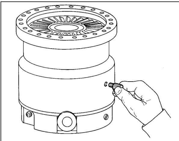
Screw the flange mod. 969-9108 on the pump, taking care of the o-ring right position.
