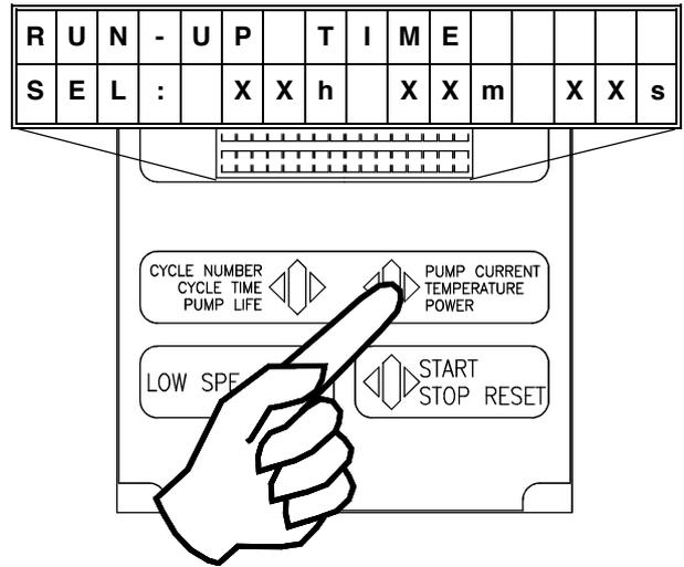
where: **RUN-UP TIME** = is the interval time from start to speed threshold value in hours, minutes, seconds. Select from 00 to 99 hours, and from 00 to 59 minutes or seconds.
