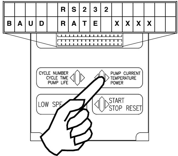
where: **XXXX** = means 600, 1200, 2400, 4800, 9600 baud rate for the host computer or printer communication. The controller is factory-set for 9600 baud rate operation.
