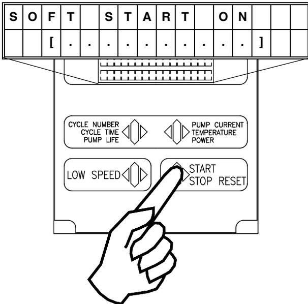
Where the sign minus (-) become a square ( □ ) when the pump finish the ramp-up step. The active step is indicated by a flashing square ( ◻ ).
