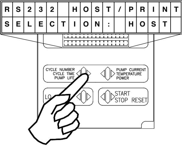
With the RS 232 connected, a bidirectional communication is established by selecting HOST. Data are sent to an external computer every time the external computer asks for the values.
