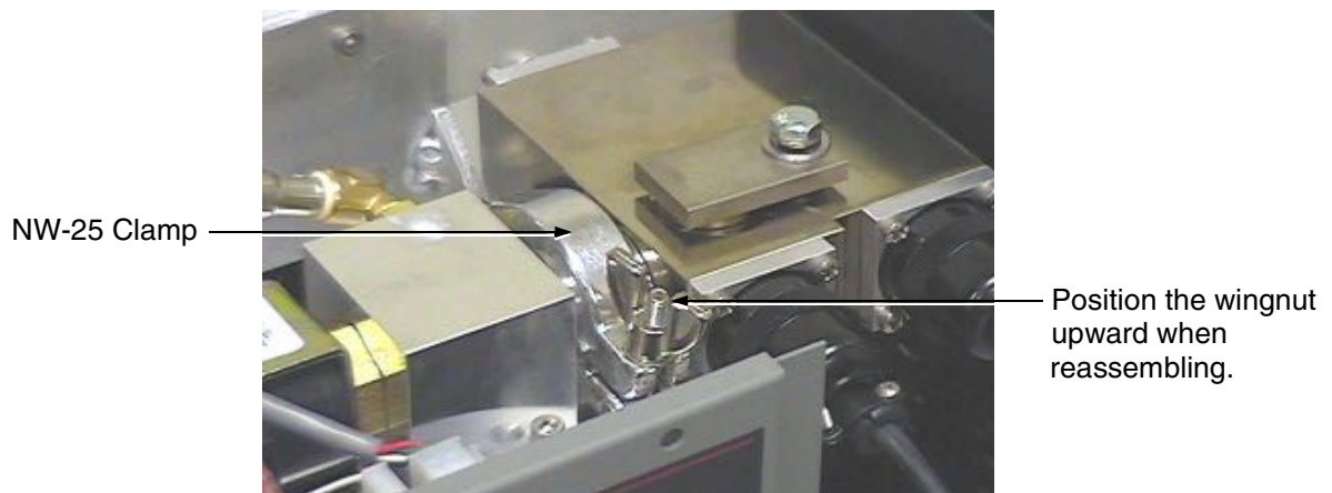
Figure 3-8 Wing Nut and Clamp
