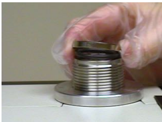
Figure 3-1 Removing the Test Port Compression Ring and O-ring
