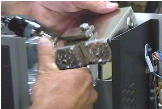
Figure 3-5 Extracting the Spectrometer Tube
