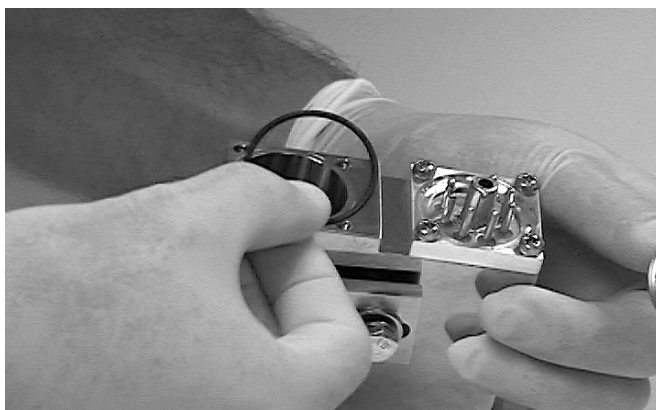
Figure 3-15 Replacing the Ion Source O-ring
