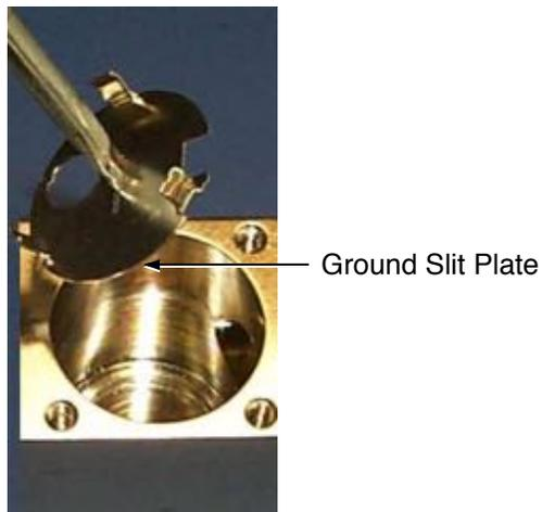
**Figure 3-12 Ground Slit Plate**
