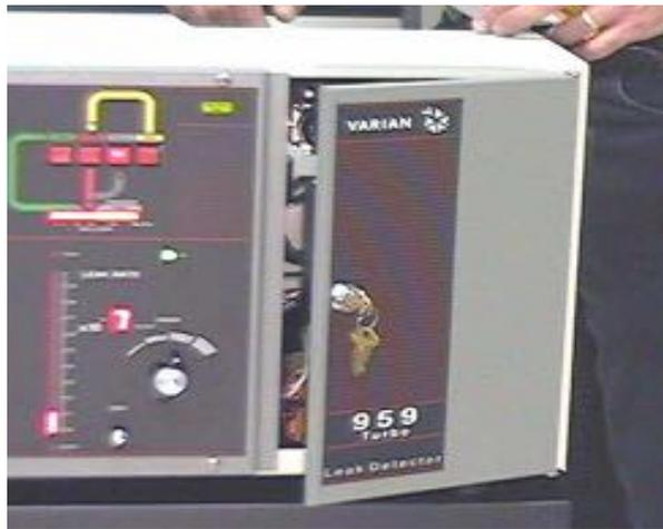
**Figure 2-3 Opening the Access Panel**
