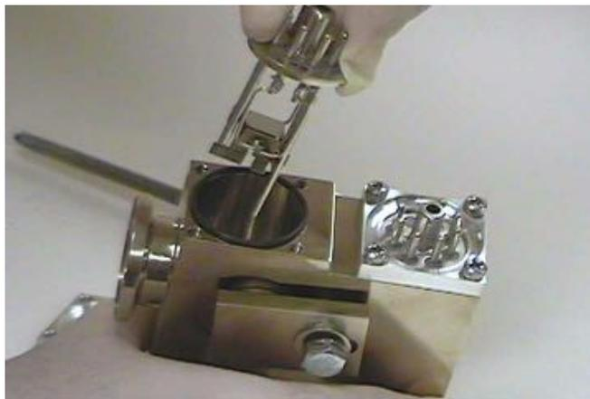
**Figure 3-9 Removing the Ion Source**
