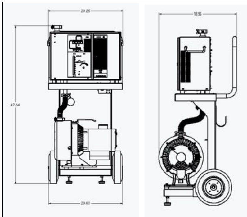
**Figure 1-1 959 Dry Pump - Front and Side**
