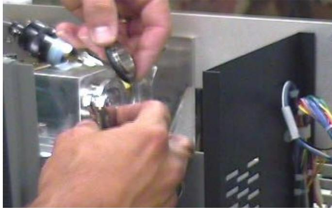
**Figure 3-6 Spectrometer Tube O-ring and Centering Ring**
