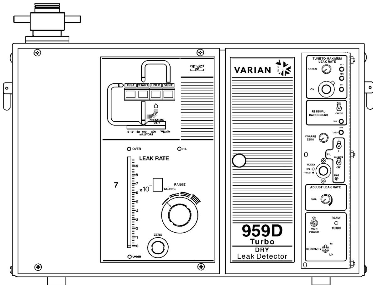
Figure 2-1 Primary (left) and Secondary (right) Controls
