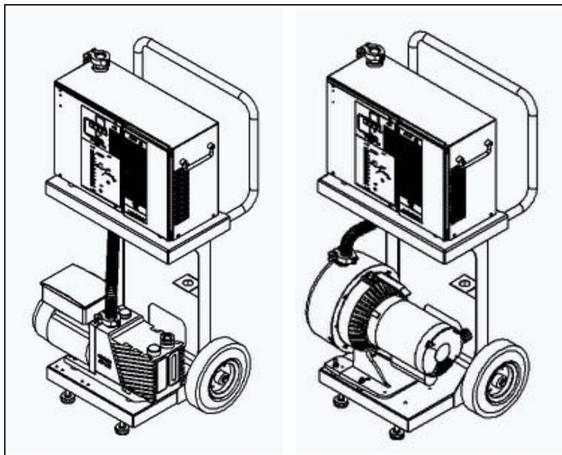
Figure 1-3 ISO View Wet and Dry Pump
