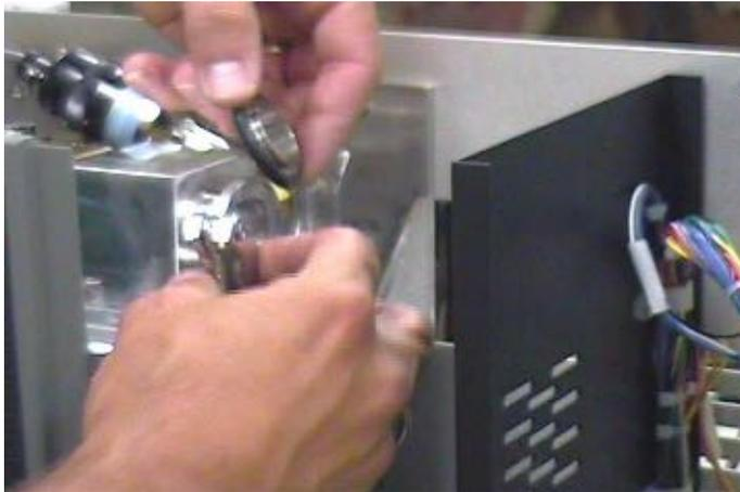
**Figure 3-18 Spectrometer Tube O-ring and Centering Ring**
