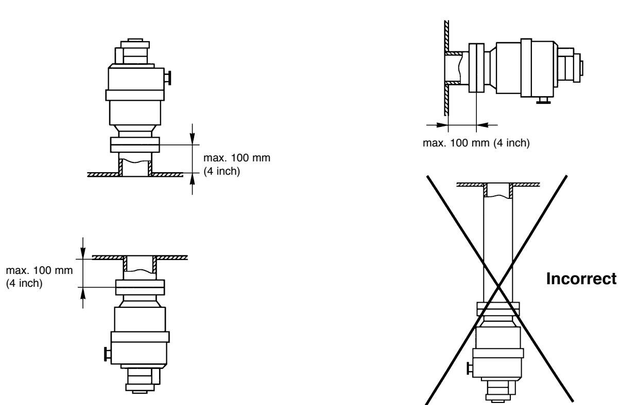
Fig. 3 Permanent flanging of the TURBOVAC to the vacuum chamber
