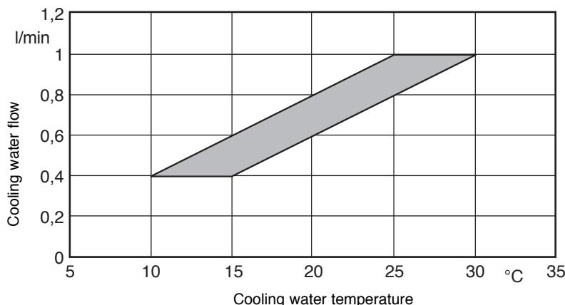
Fig. 5 Cooling water consumption
