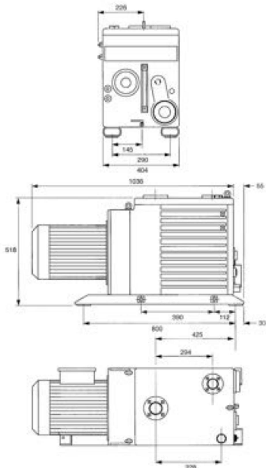
Figure 3 - Dimensions EIM2755 and E2M2755 (mm)
