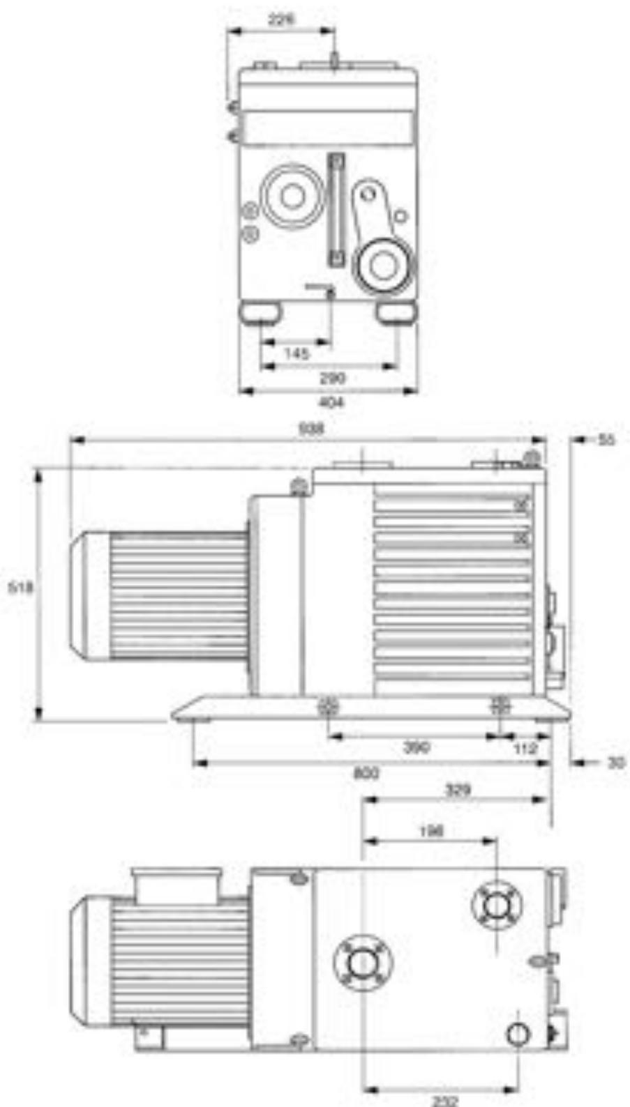
Figure 2 - Dimensions E1M175S and E2M175S (mm)
