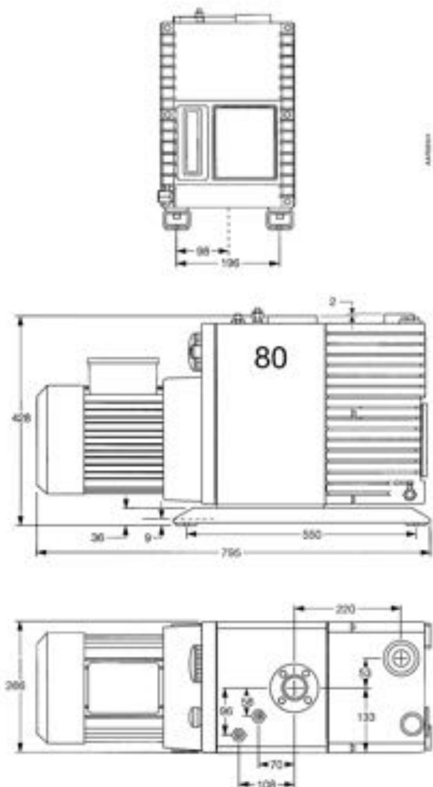
Figure 3 - Dimensions E1M80 and E2M80 (mm)
