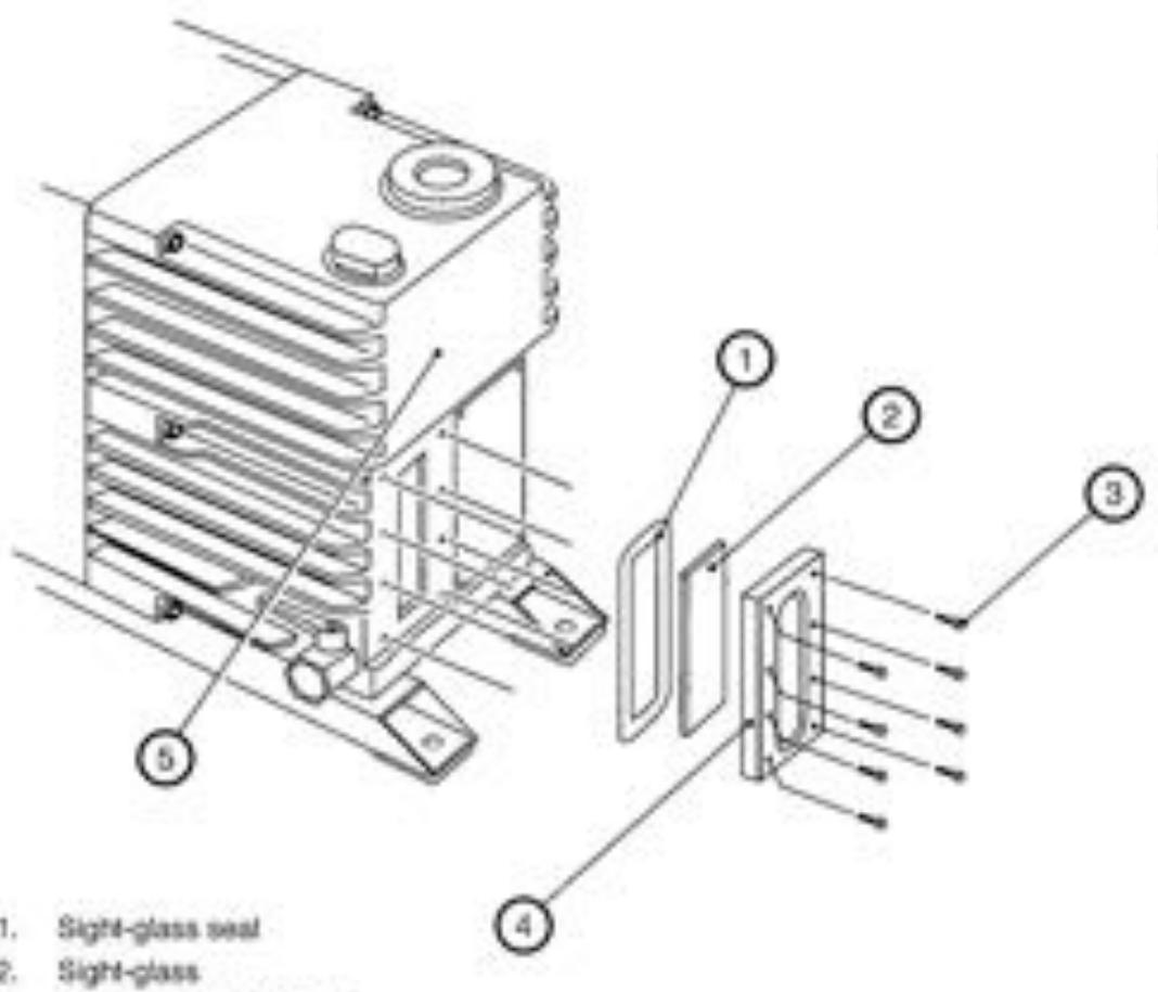
Figure 11 - Oil-level sight-glass assembly
