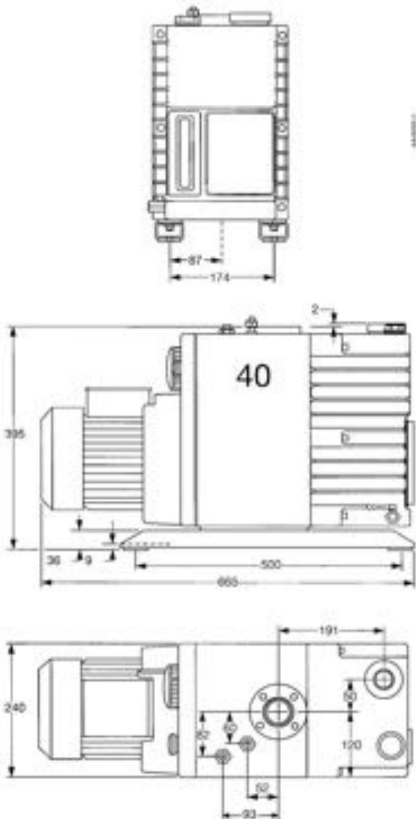
Figure 2 - Dimensions E1M40 and E2M40 (mm)
