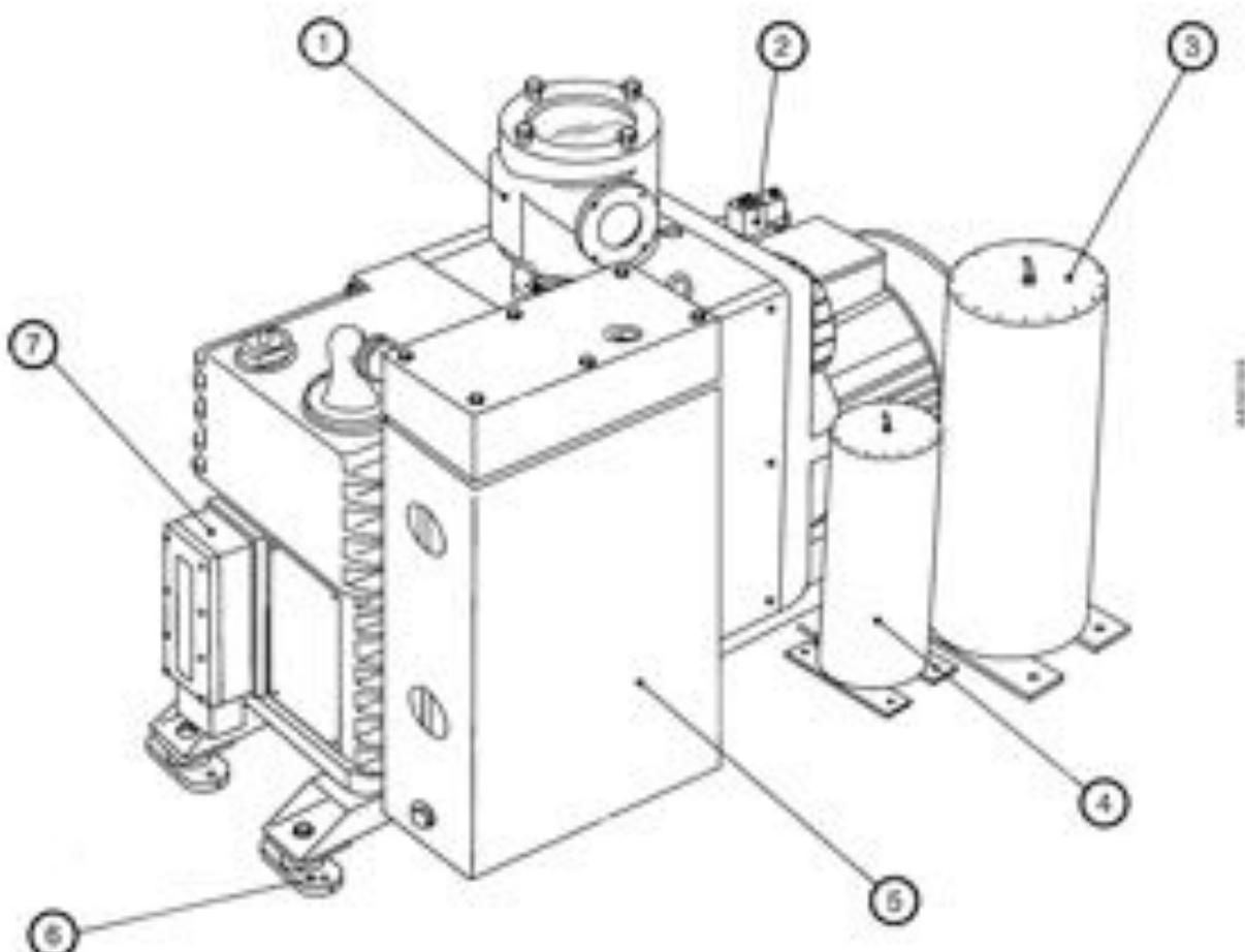
1. Inlet dust-filter or inlet catchpot or inlet chemical trap or high capacity inlet dust-filter
