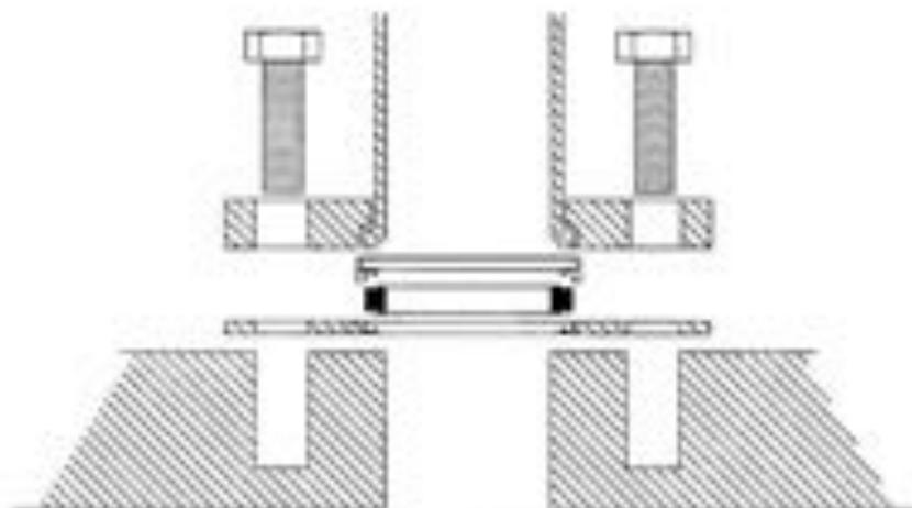
Figure 8 - Connect inlet to NW40 inlet fittings
