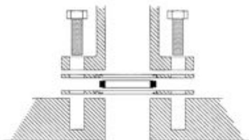
Figure 7 - Connect inlet to ISO40 fittings
