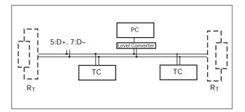
All units connected to the bus must have differing serial interface addresses (parameter 797).
