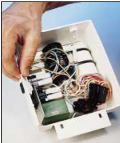
High/low voltage configuration with changeover switch
