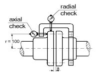
When using dial gauges for the alignment, proceed as shown in the diagram.
