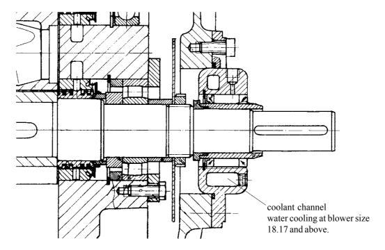
The radial sealing rings run on a hardened and ground shaft protection sleeve. The oil chamber ensures that the radial sealing rings are vacuum-tight and have a long service life.
